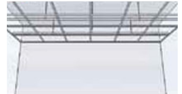
6. CROSS T-BAR CONSTRUCTION
